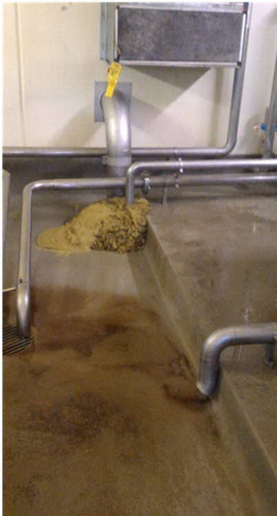
Figure 9. Dry hopping with the Iso-Mix external drive: effective removal of hop solids during centrifugation.
