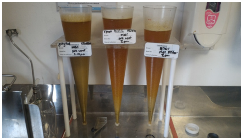
Figure 5. Carryover of hop solids through prefiltration centrifuge.
