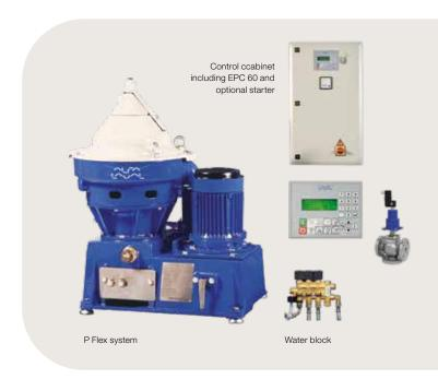
A P Flex module is a compact separator module that can be built to a customer-specified configuration from a wide range of modular skids and blocks, including any type of heater and a sludge removal kit. Multi-modules are possible, as well as mixed modules including one or more P separators for the simultaneous treatment of different types of mineral oils. All P Flex modules are factory tested to ensure faster start-up and commissioning.
