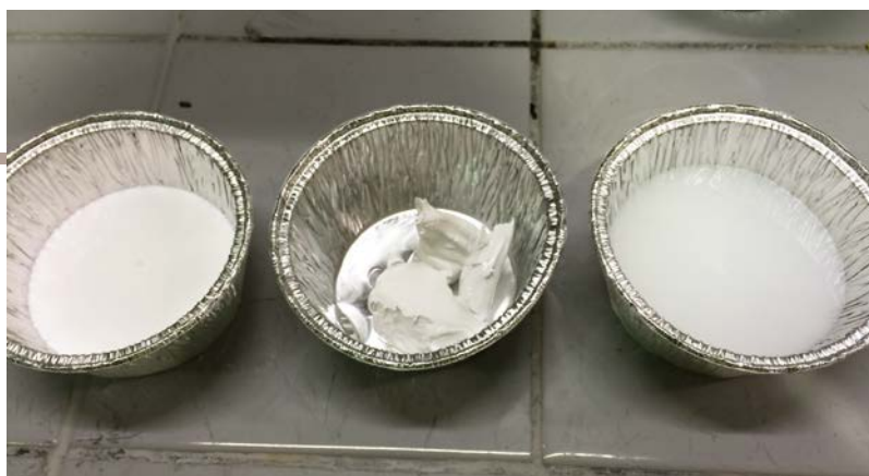
Samples from a dewatering test on calcium carbonate. The inlet slurry (left) is separated into the solids fraction (middle) and liquid fraction (right) in an Alfa Laval decanter centrifuge. Parameters such as bowl speed, pond level setting and differential speed can be changed in the decanter to meet targets for solid-fraction dryness, particle size and separation efficiency.
