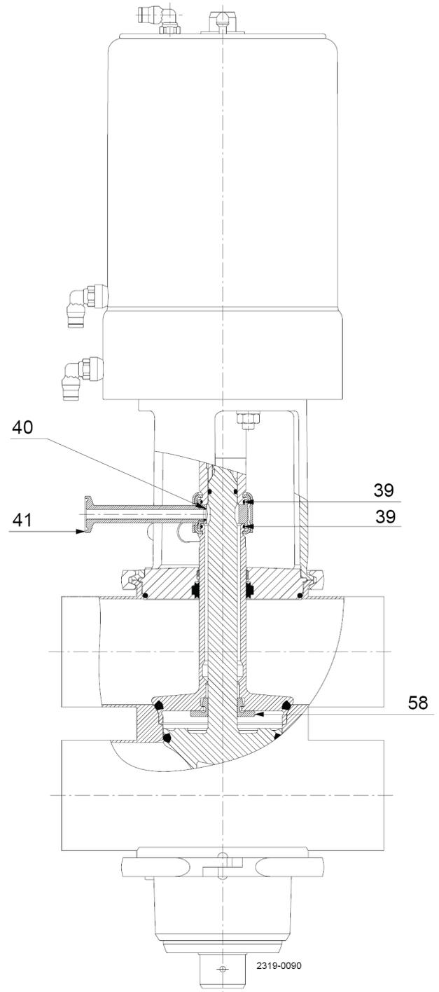
with SpiralClean in leakage chamber
