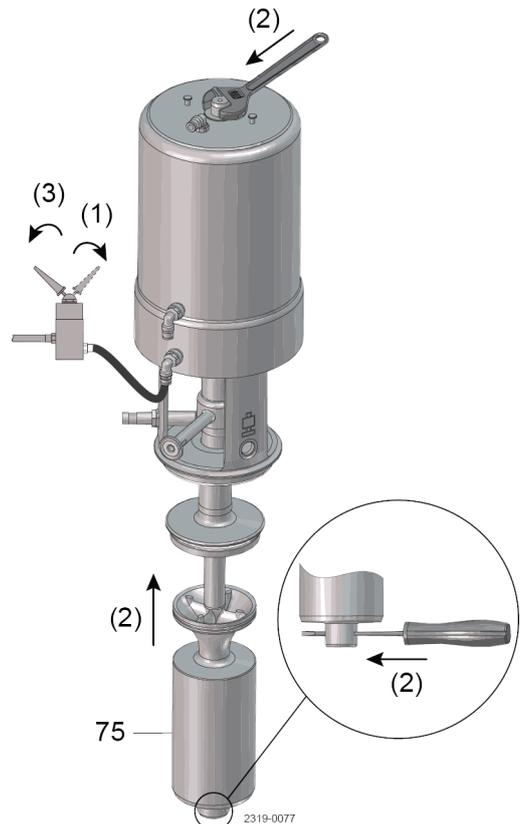
The valve is designed so that internal leakages do not result in the products becoming mixed.
