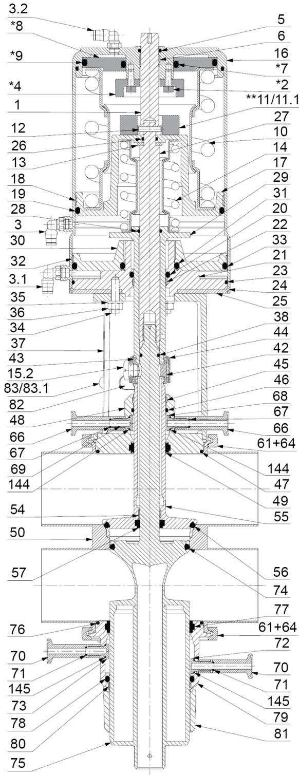
without SpiralClean in leakage chamber
