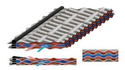
The recently launched Alfa Laval WideGap 100 gasketed plate heat exchanger was specially designed for handling media with coarse particles, fibres and solids. The wide, corrugated channels let dirty fluids pass freely and helps avoiding clogging, reducing fouling and increasing heat transfer. WideGap 100 is ideal for industrial waste treatment eg. effluent concentration, waste reduction and product recovery for those aiming for Zero liquid discharge.
