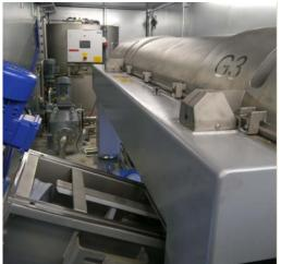
At IFAT 2016 Alfa Laval presents a complete containerized ALDEC G3 Decanter system equipped with everything to run field tests for cost- and energy efficient thickening and dewatering of municipal and industrial sludge.
