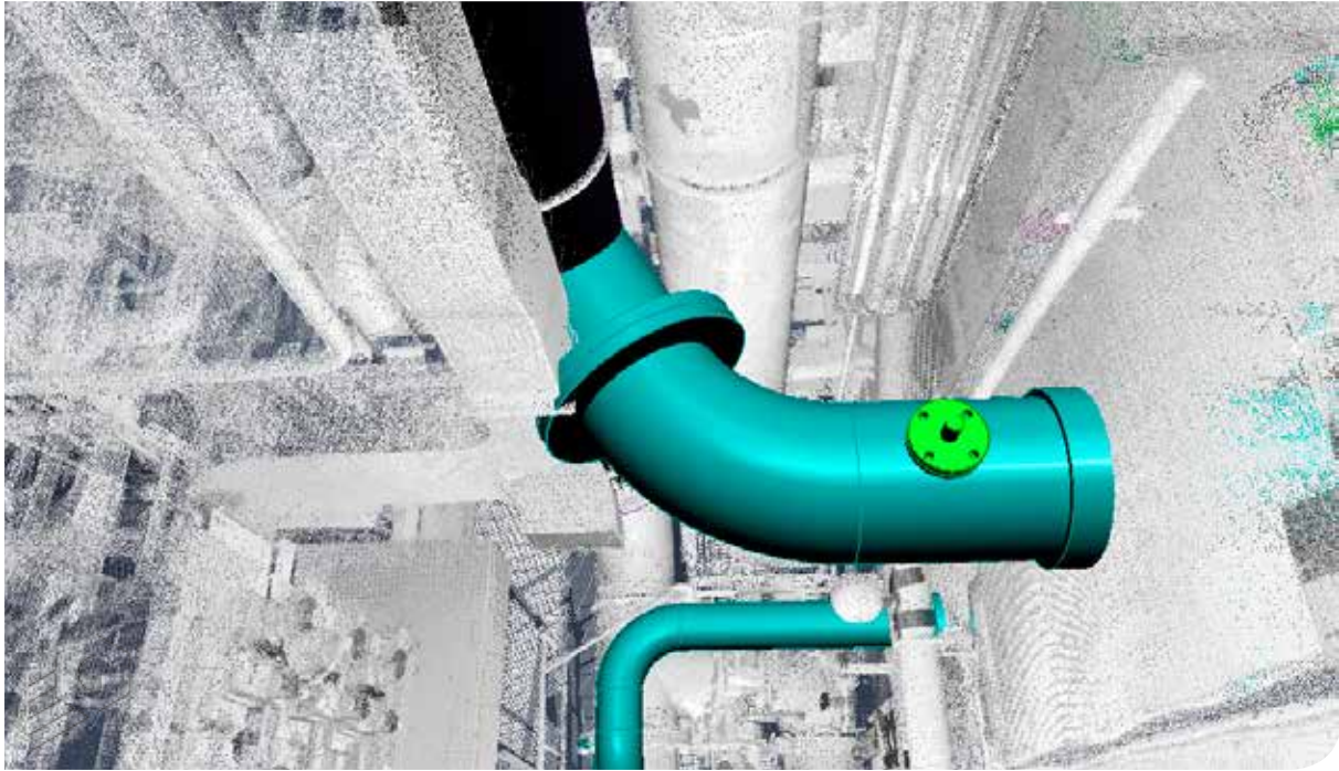
A 3D visualization demonstrating how new ballast piping would interfere with the existing ventilation duct
