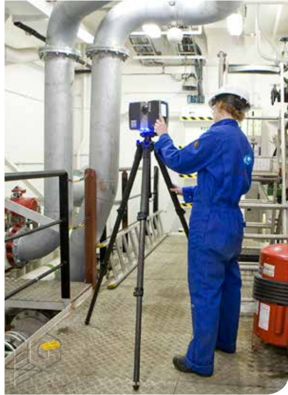
Onboard survey and 3D scanning
