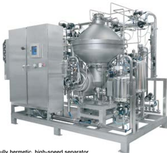
Culturefuge is a fully hermetic, high-speed separator developed for applications involving mammalian cell cultures and other sheer-sensitive biological material.
