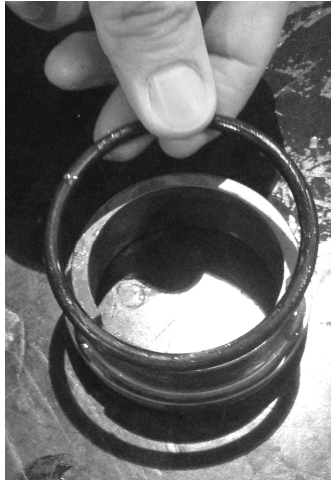
Figure 11, O-ring for stationary part of seal
