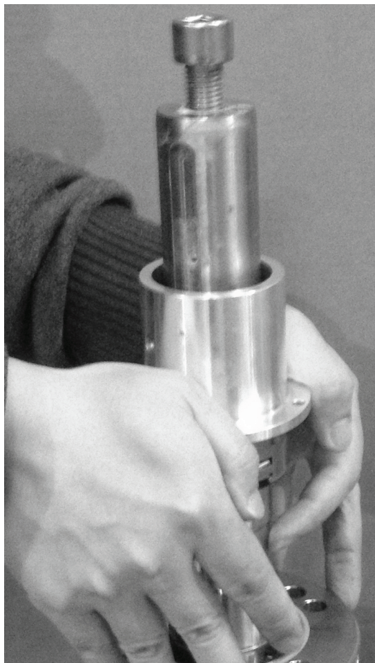
Figure 10, Pressing down the seal
