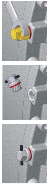
Figure 3-2: Removing vent plug and fitting the pressure vent
