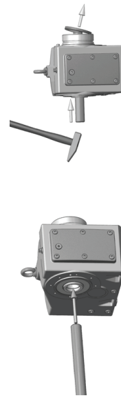
Figure 3-5: Removing the factory-fitted closing cap
