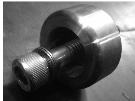
Figure 15, Bushing for shaft / gear motor
