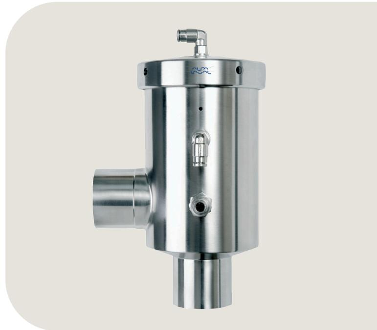
Air pressure exerted on the lower portion of the membrane set forces the SB Pressure Exhaust Valve open. The valve is now fully cleanable either by an optional CIP supply valve, supplying CIP to the cleaning nozzle on the valve housing, or cleaning along with rest of the installation with a separate CIP line.
