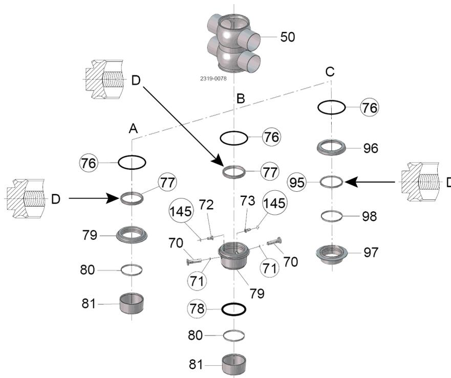
D = Lubricate with Alfa Laval Lubricant on ID
