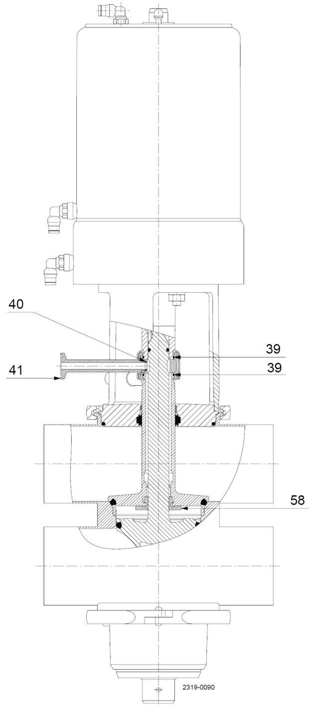
with SpiralClean in leakage chamber
