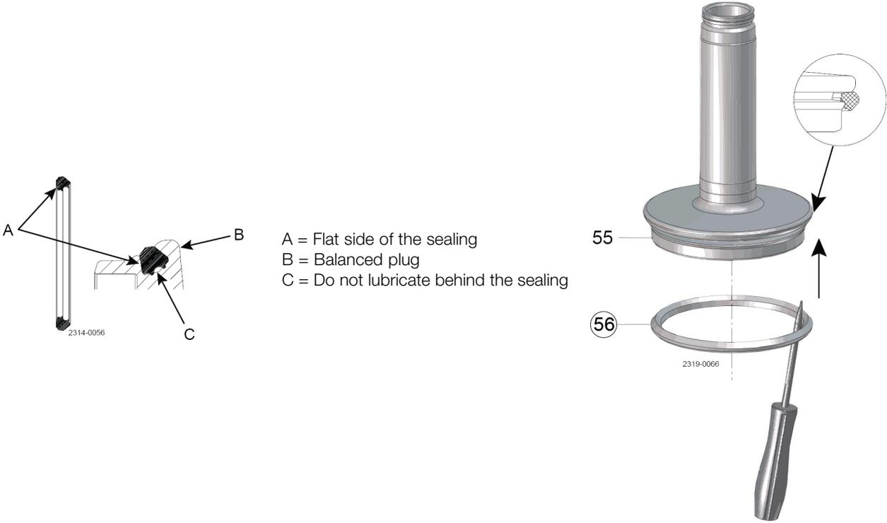
Carefully lubricate sealings with suitable soap or lubricant (Alfa Laval Lubricant), before pre-mounting.
