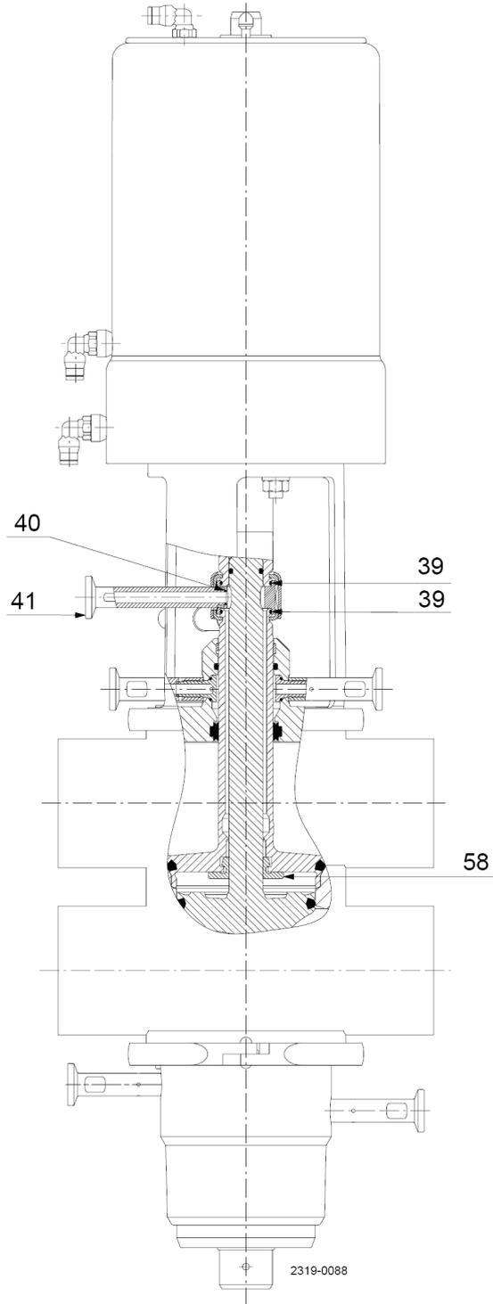
with SpiralClean in leakage chamber
