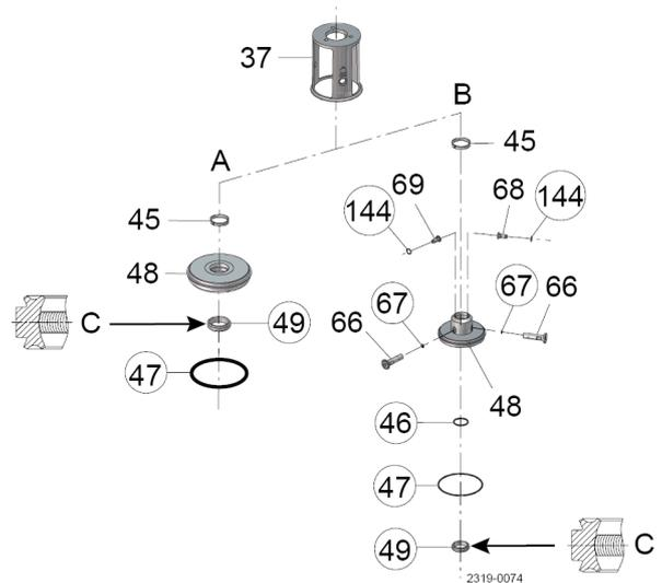
C = Lubricate with Alfa Laval Lubricant on ID
