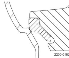
Figure 3. PTFE plug seal (TR2)
