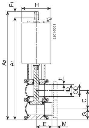
Figure 1. Shut-off valve
