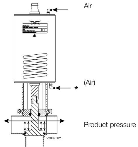
\* Careful if using support air on spring side and a high product pressure above the plug, as this can result in a high "hammer effect" which can damage the actuator.
