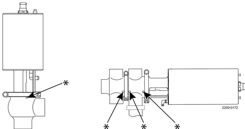
\* = Leakage detection hole
