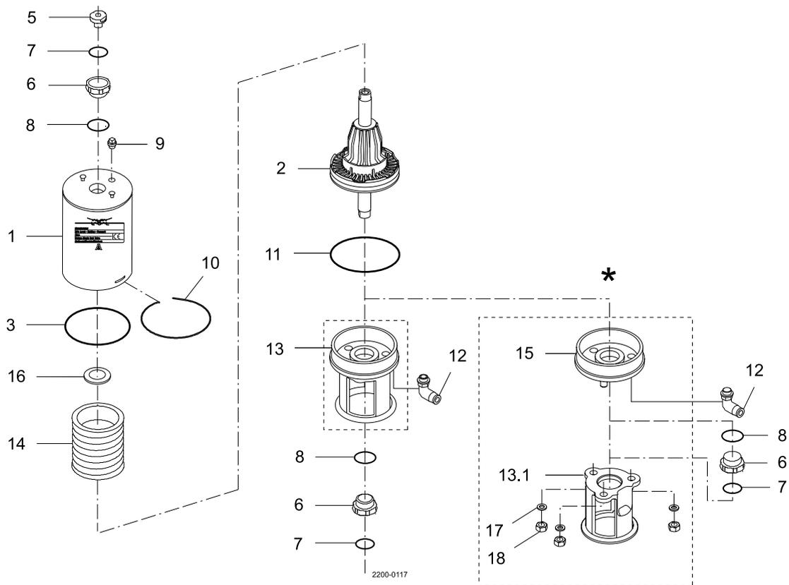
\*) "Removable yoke with bolts" version, produced from 2006 to June 2016.
